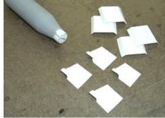
For each set of bomb halves, there is a doubler half. This part is marked with a centerline. Cut along the centerline to form two doublers.
