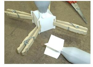
The fins and box edges have been formed slightly oversized so they could be trimmed after the adhesive has dried completely. Scissors can be used for the rough trimming however; sandpaper should be used to produce a clean edge.
